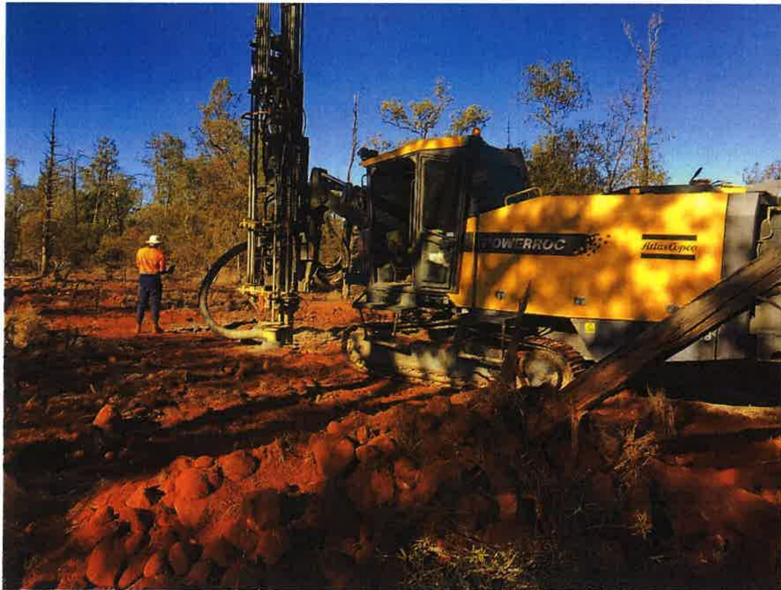
Plate 1 – Atlas Copco (Epiroc) T35 tophammer rig drilling on Tikitere East ridge line. Thin veneer of residual basaltic soil and basalt cobbles can be seen pushed up in foreground.
