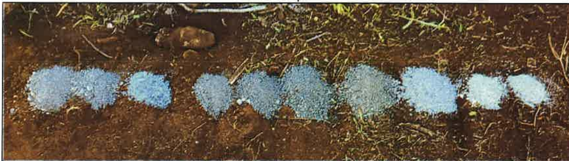
Plate 4 – Rock Chips from TR18 drilled on western basalt ridge. Shows 8m of slightly to distinctly weathered basalt followed by 2m of sandstone. Top of hole on left.
